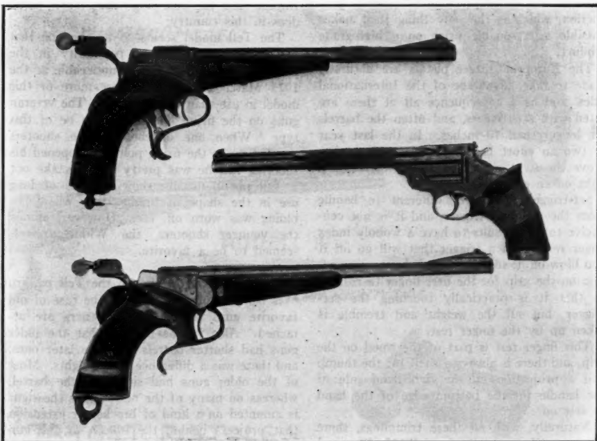
Top—Hartmann; Middle—S. & W.; Bottom—Widmer. Note How Right Side Grip is Carried Forward to Form Rest for Trigger Finger
